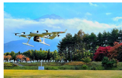
A high-performance eVTOL fixed-wing drone, manufactured by Wingcopter GmbH of Germany, equipped with an unmanned aerial vehicle-mounted YellowScan Voyager scanner (Photo courtesy of ITOCHU Corporation)
