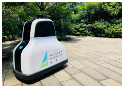
The cocobo autonomous security robot can patrol on public roads during the day and at night
