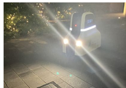
The cocobo autonomous security robot can patrol on public roads during the day and at night
