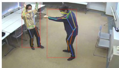
Example of human behavior (threat) detected by the SECOM AI Behavior Detection System
