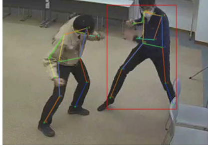
Actions detected by the SECOM AI Behavior Detection System include altercations (left) and falls (right)
