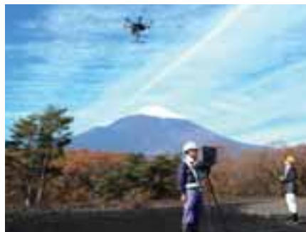
3D terrain models created using data collected by drones (i-Construction project)
