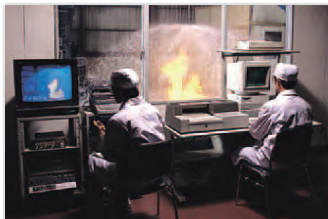
Test of low-expansion foam fire extinguishing system (Nohmi Bosai)
