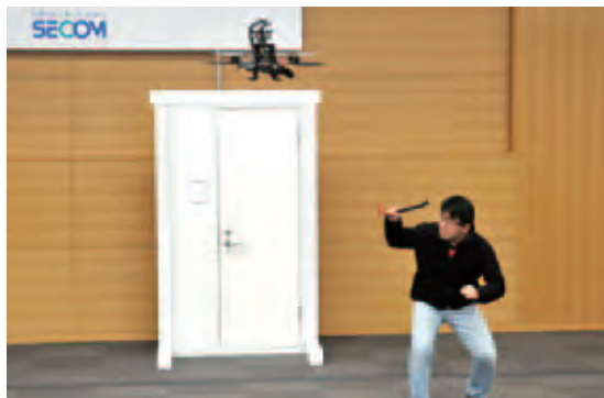
The robot takes off autonomously and flies toward intruders
