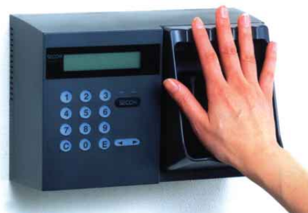
SESAMO IDj, an access-control system that identifies individuals by the veins in their hands
