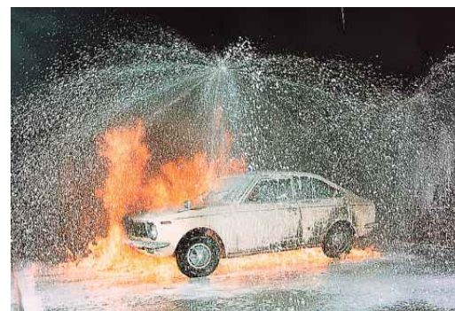
Foam fire extinguishing system
