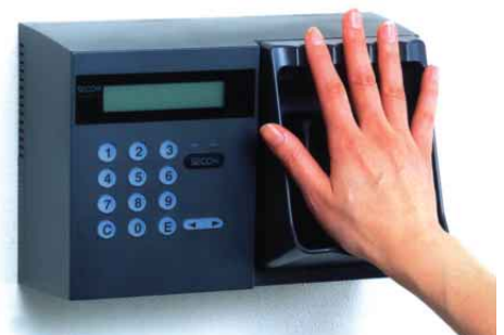
SESAMO IDj, an access-control system that identifies individuals by the veins in their hands
