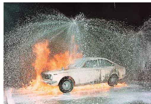
Foam fire extinguishing system
