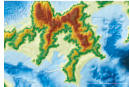
Aerial laser surveying facilitates seamless 3D topographical measurements above and below water
