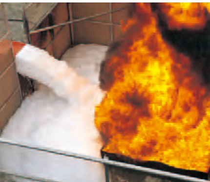
Test of a high-expansion foam fire extinguishing system (Nohmi Bosai)
