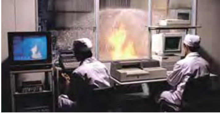
Test of low-expansion foam fire extinguishing system (Nohmi Bosai)
