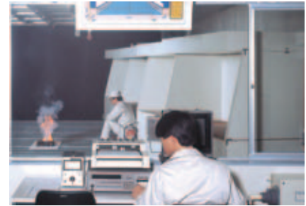
Testing of fire extinguishing system
