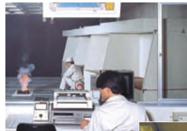
Clean room testing of fire extinguishing system
