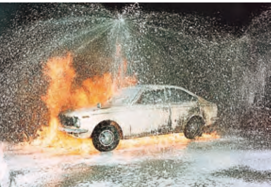
Foam fire extinguishing system
