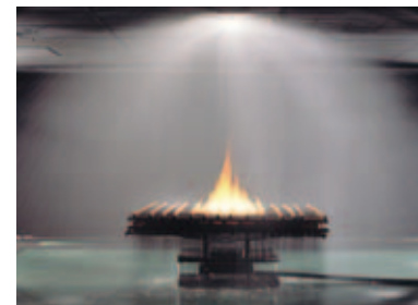
Test of sprinkler system
