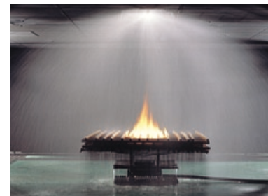
Test of sprinkler system
