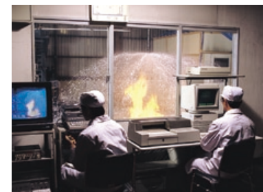
Test of foam fire extinguishing system
