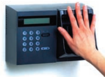
SESAMO IDj, an access-control system that identifies people by the veins in their palms
