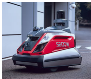
SECOM Robot X outdoor surveillance robot
