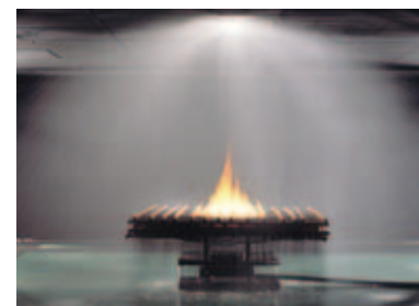
Test of sprinkler system
