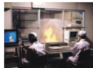
Test of foam fire extinguishing system
