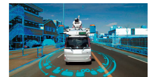
Real Dimension vehicle-mounted 3D road condition surveying system
