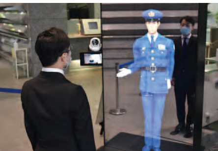
Trial using the Virtual Security Guard System to measure visitors' body temperature
